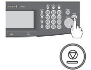
• To return the machine to the initial screen of the current active mode.
